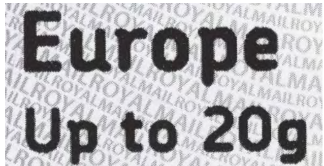
Gravure printed version with screening dots clearly visible
